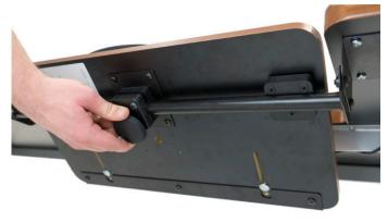
To tilt your tray, loosen the knob under the tray and tilt the platform to your desired angle. Then re-tighten the knob.
