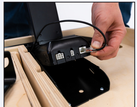
3. Connect Hand Controller Cable
