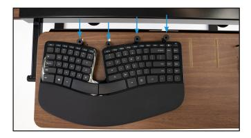
3. Slide the rubber bumpers forwards or backwards to find a comfortable depth for your keyboard.
