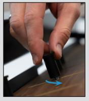
2. To loosen the rubber bumpers, hold the screw underneath and twist counterclockwise.
